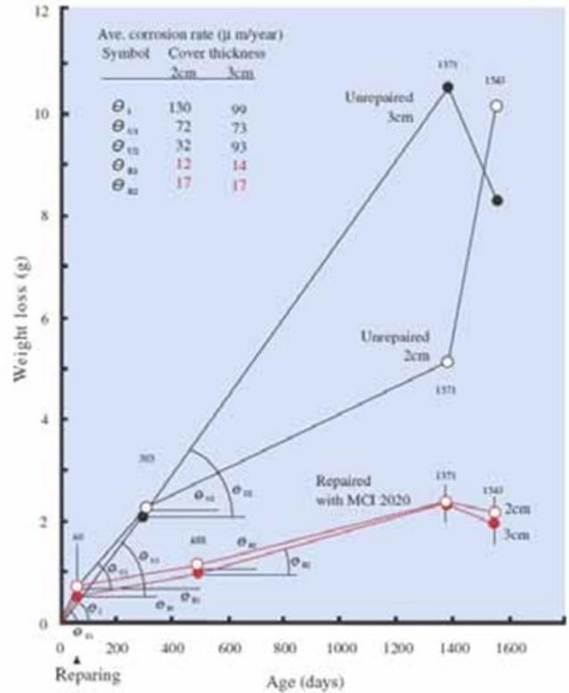
MCI-2020 treated specimens decreased the amount of corrosion up by ½ to 1/6 that of the control samples. When applying MCI-2020 after cracks appeared, it worked very well in reducing corrosion rates in samples. Study used ASTM G109 sized beams cast with 3 rebar in a triangular array. Chloride solution was ponded on the surface for 2 weeks of a 4 week test cycle. Half-cell potentials and corrosion current readings were taken monthly.
